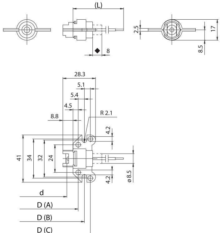
◆ Maximum jut of the steatite body during lamp insertion
