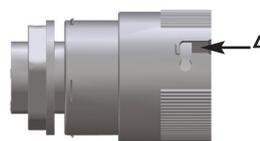
3702/V...: socket (3) with holes for fixing (4) and gland
