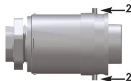
3701/M...: plug body (1) + shell with fixing pins (2) and gland
