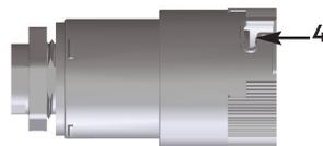
3702/M...: socket (3) with holes for fixing (4) and gland
