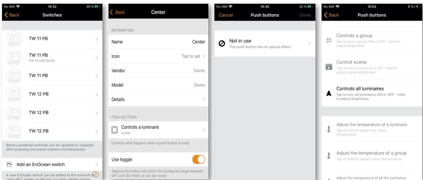
If the Control scene or Cycle scenes option is used, you can also Disable dimming. Disabling dimming prevents a long button push (or the +/- buttons on the Xpress) from adjusting the scene dimmed level.
