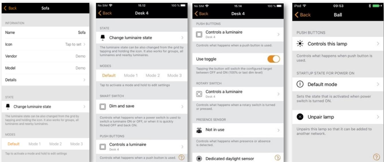
**PUSH BUTTONS** and **ROTARY SWITCH** Allow you to select the function of a luminaire's inbuilt switch (if fitted), depending on the type of Casambi device which is being used. For detailed information about push buttons please see the Push buttons section in the Appendix.
