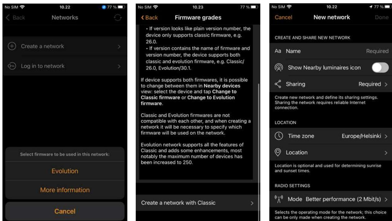
The network Radio settings have four Mode options. These determine the communication speed and potential communication range for devices in the network.
