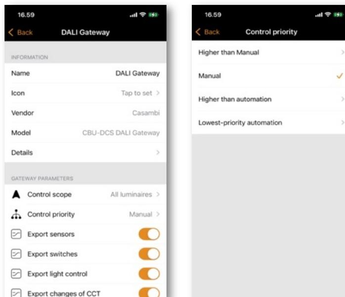
Input dimming curve defines how the dim levels that the DALI system sends to the Casambi DALI Gateway are interpreted and sent further within the Casambi network.
