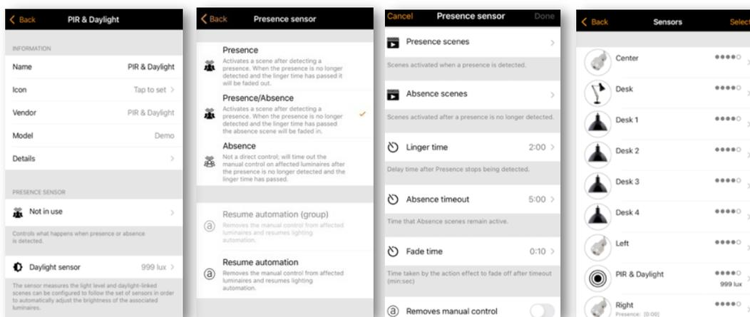
A presence sensor will display a 'walking person' icon in the top right of the main sensor icon image when presence is detected.
