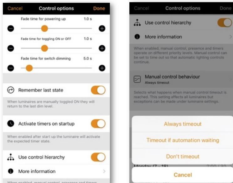
**Manual control fade out** This option sets the time within which a luminaire fades out once manual control has expired.
