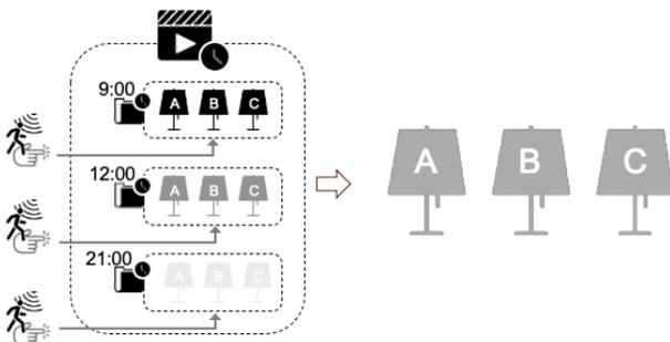
*Each condition scene will trigger as expected (e.g., 3 luminaires will dim as expected)*
