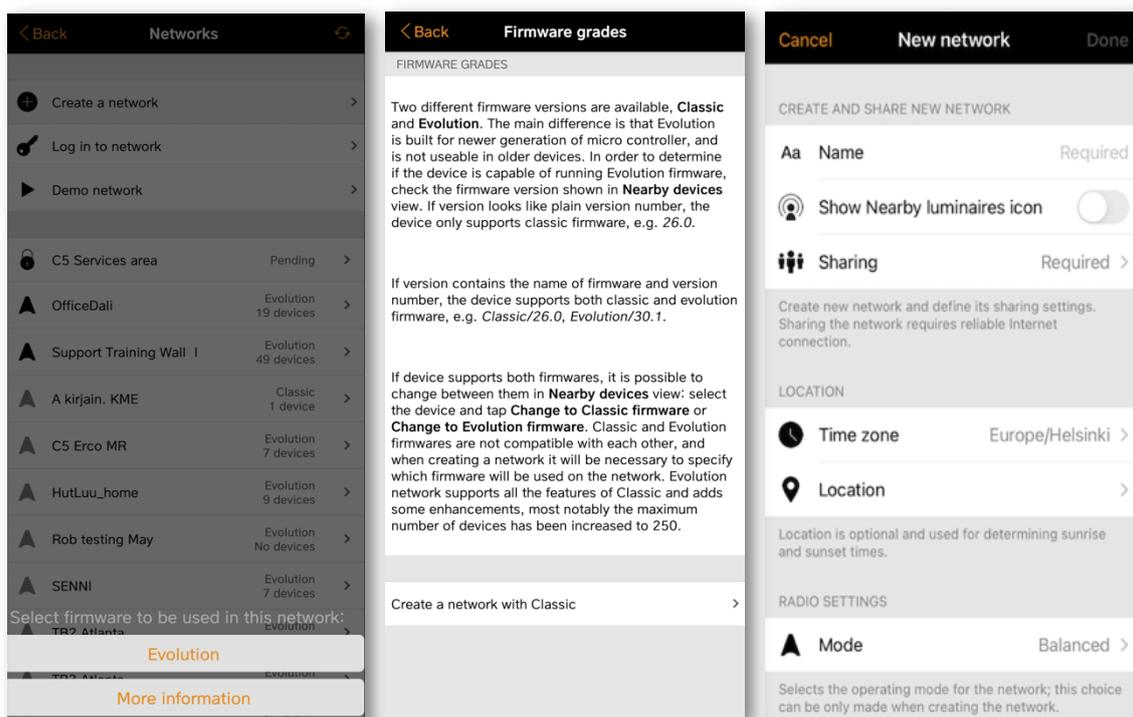
The network Radio settings have four Mode options. These determine the communication speed and potential communication range for devices in the network.
