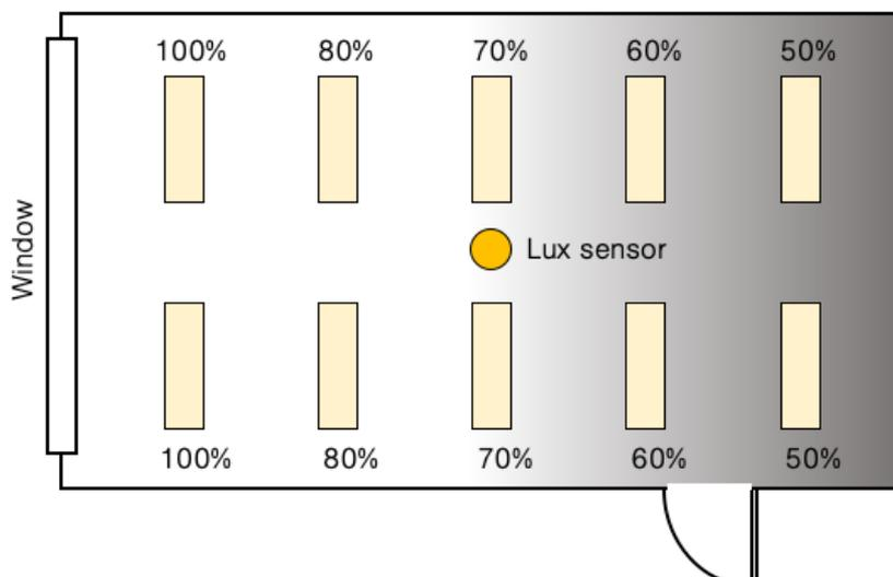
If you wish, you can define a separate daylight gain for each luminaire in a Casambi network. By default, the daylight gain for luminaires is set to 100%.
