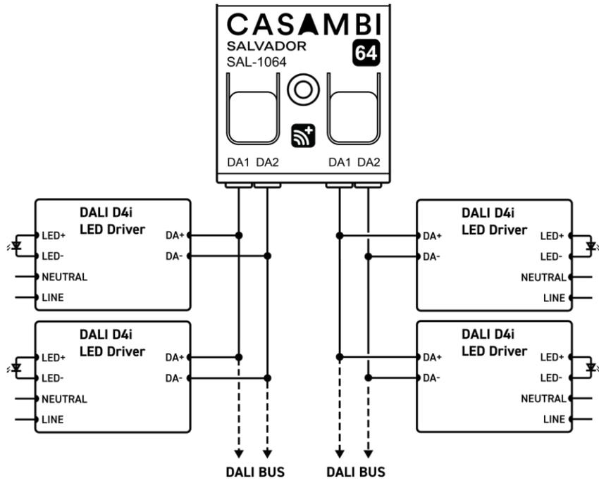
Do not exceed 250 mA bus current. Observe bus polarity.
